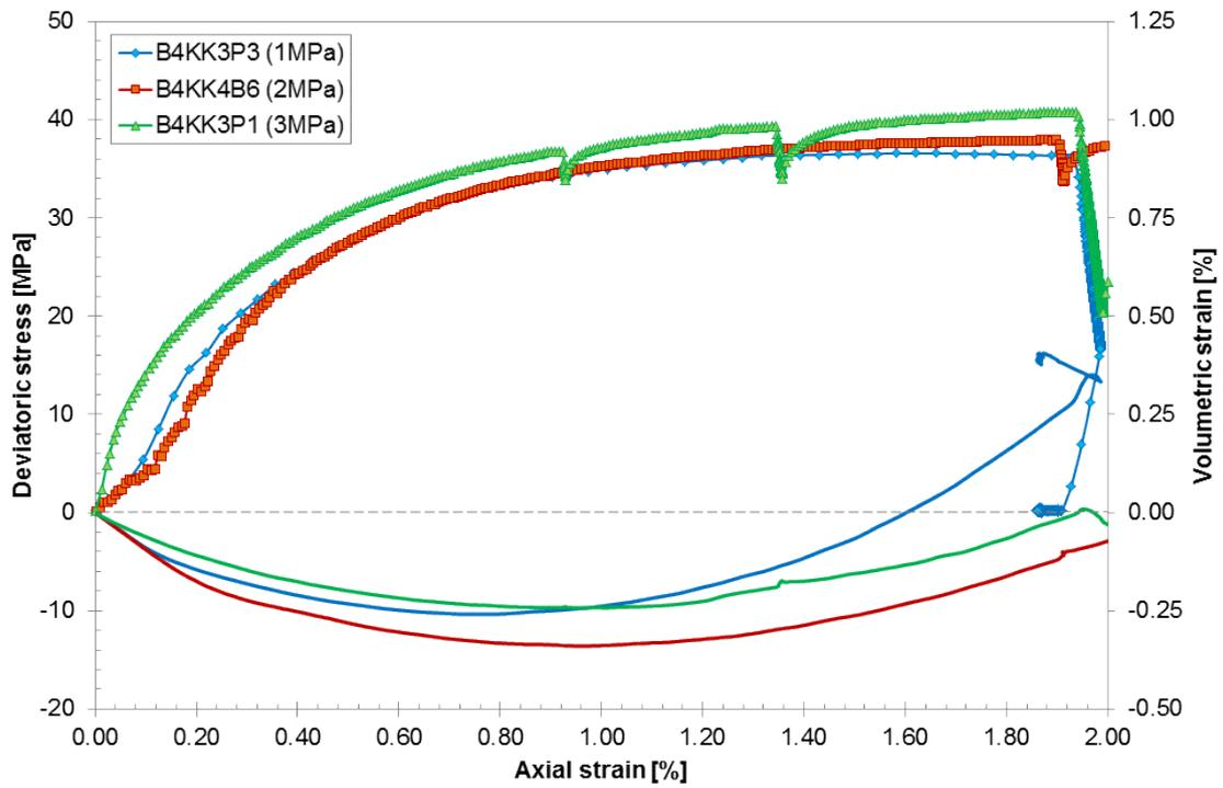
**Fig. 3.9** Stress-strain curves obtained on the salt concrete samples at different confining stresses
