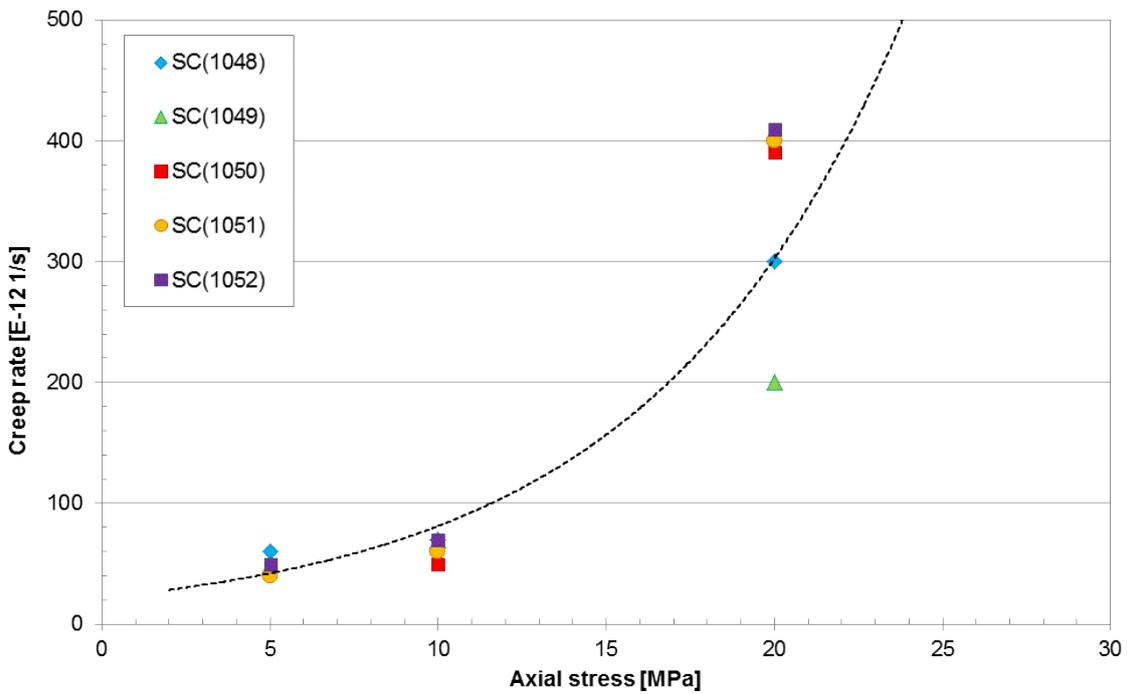
**Fig. 3.19** Steady-state creep rates obtained on five salt concrete samples as a function of applied uniaxial loads
