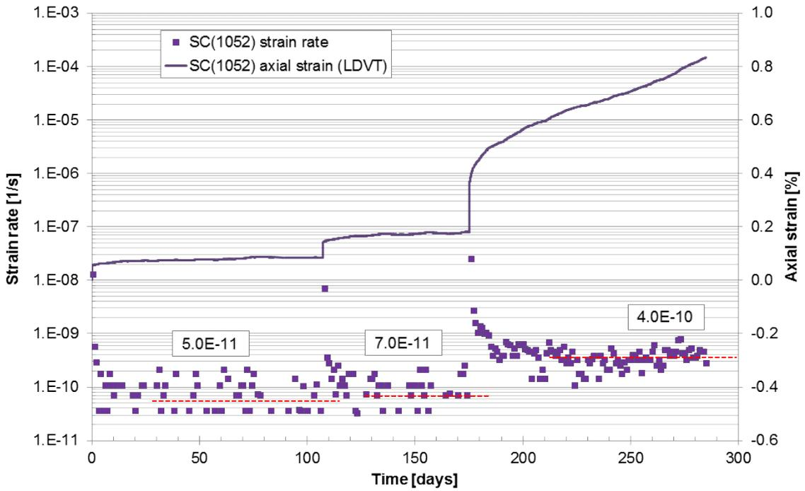
**Fig. 3.18** Long-term uniaxial creep behaviour of salt concrete sample no.1052 under multi-step loads – axial strain and derived creep rates
