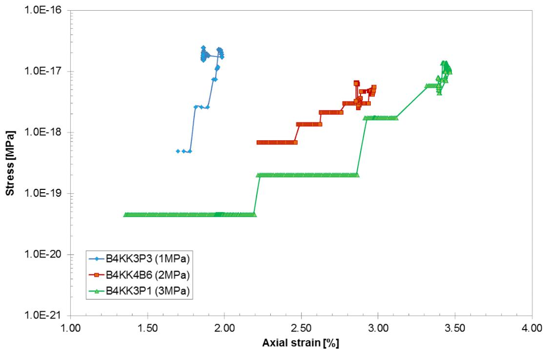
**Fig. 3.10** Strain-permeability curves obtained on the salt concrete samples at different confining stresses
