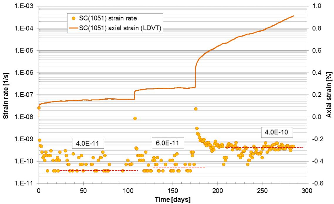
**Fig. 3.17** Long-term uniaxial creep behaviour of salt concrete sample no.1051 under multi-step loads – axial strain and derived creep rates
