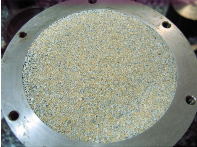
**Figure 18: Appearance of the bottom part of sample MGR19 after compaction**
