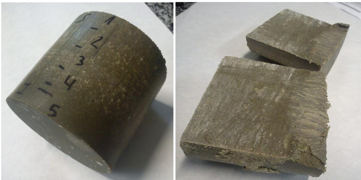
**Figure 24: Subsampling sections for sample MGR17 and internal appearance after longitudinal cutting**
