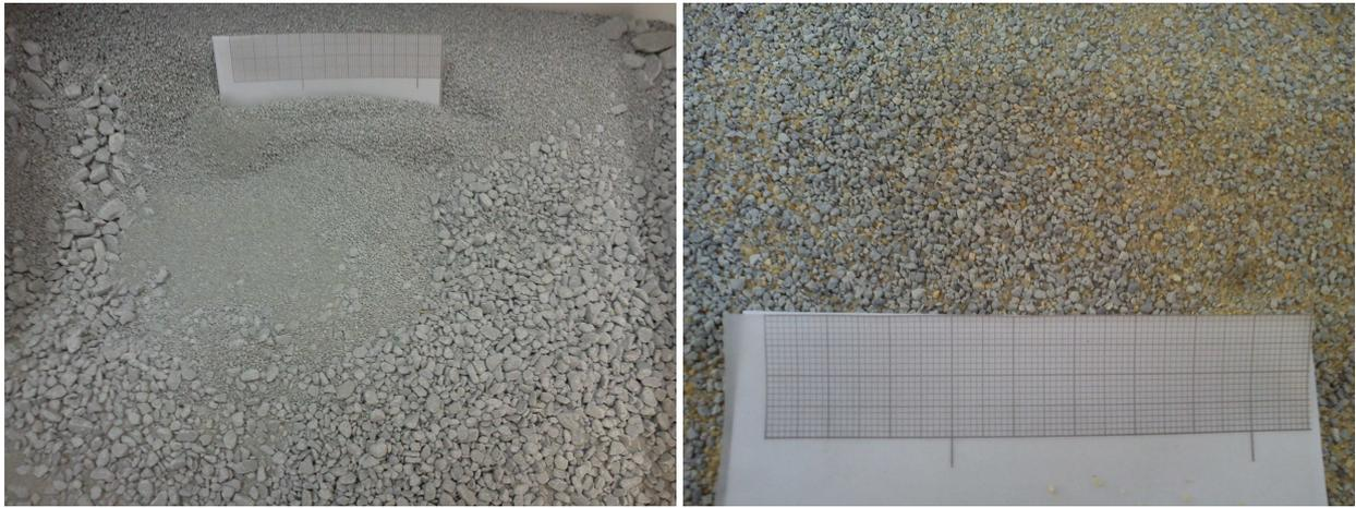
**Figure 2: Appearance of the materials received at CIEMAT: MX-80 pellets (left) and sand/bentonite mixture (right)**
