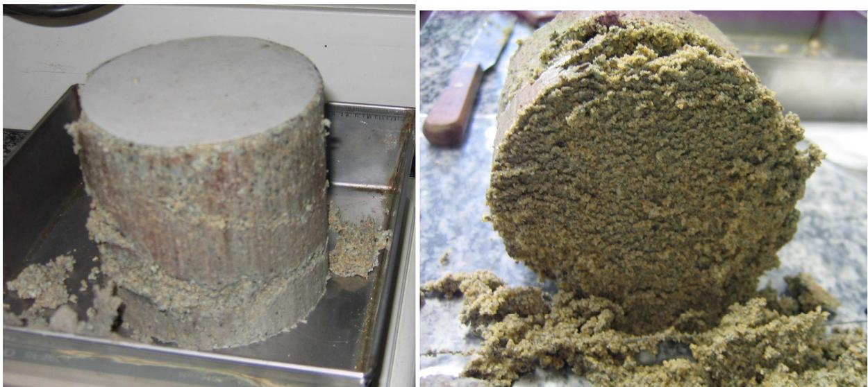
**Figure 11: Appearance of sample MGR15 after extraction**
