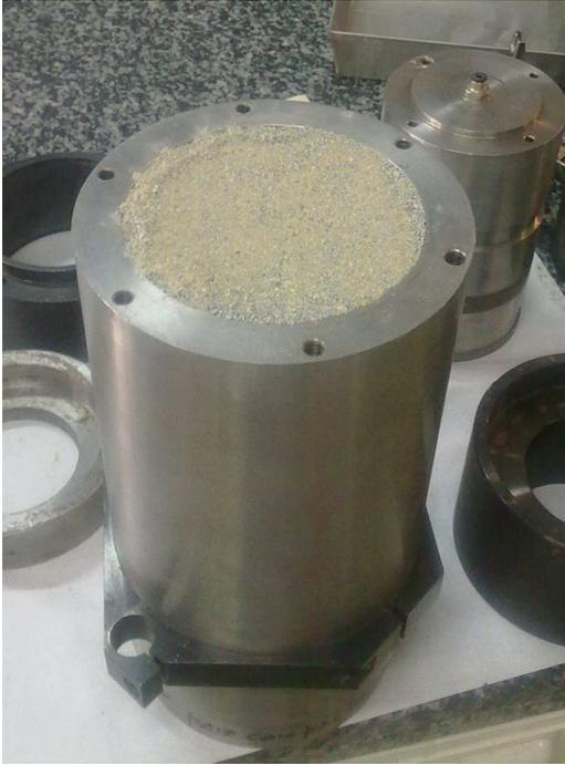
**Figure 13: Appearance of the bottom part of sample MGR16 after compaction**
