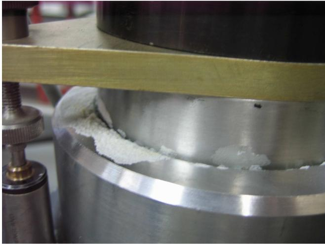
Figure 8: Salt precipitate in the upper part of the oedometer caused by the filtration of water in test MGR15
