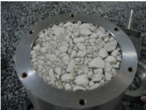
**Figure 13: Appearance of sample for test MGR13 after compaction**
