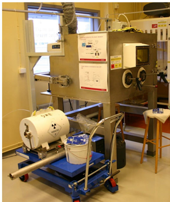
Figure 3: The laser ablation hot cell and the sample transfer cask
