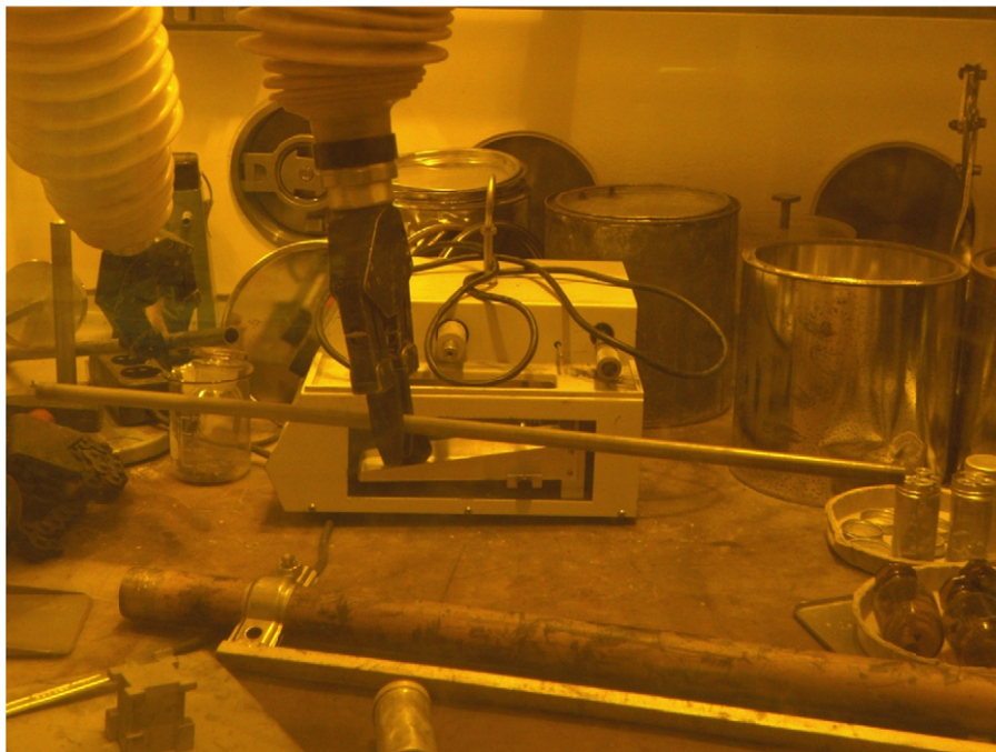
Figure 1: 50.4 GWd/t HM PWR fuel rod segment after removal from the lead shield storage tube at the shielded box-line of KIT-INE before transport to JRC-ITU
