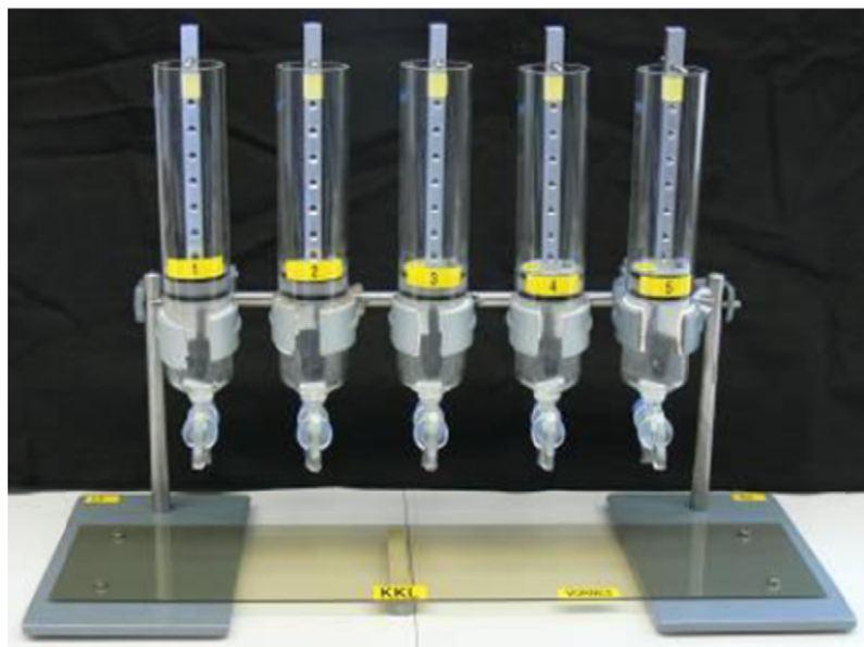
Figure 1: Experimental setup used by PSI for the leaching of the spent fuel, and applied also at SCK•CEN [Courtesy of PSI]
