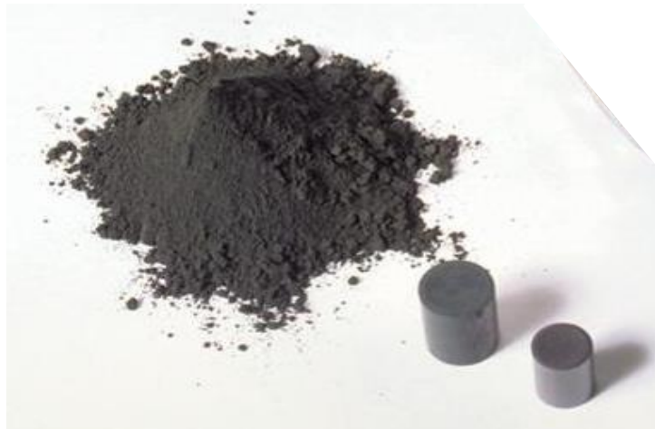
Figure 1. From powder to pellet. A) Powder: \text{UO}_2 grain size of 20\text{ }\mu\text{m} ; B) Pellet: PWR 17\times 17 - \varnothing 8.17 (AREVA) - a length of 9.8\text{ mm} , BWR 10\times 10 - \varnothing 8.87 (Atrium 10XP) - a length of 10.5\text{ mm} .
