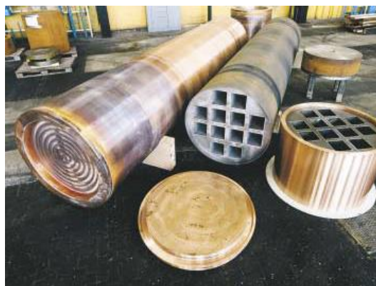
Figure A - 1. Components of the Swedish canister concept at SKB's Canister Laboratory in Oskarshamn.
