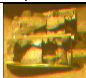
Cladding plus adhered residues that have not been separated in the cutting and extraction process prior to the experimental tests.
