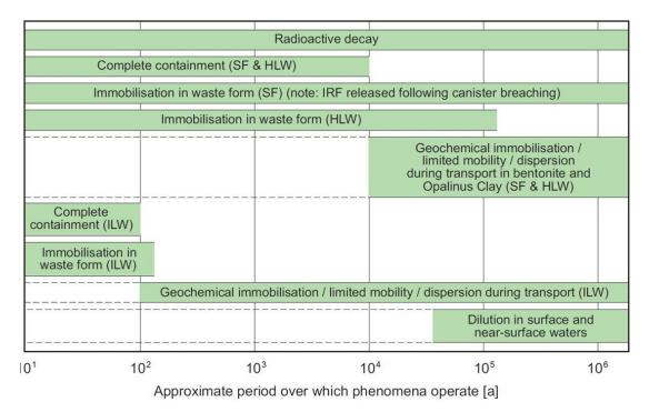
**Figure 3.2:** Key processes (phenomena) contributing positively to long-term safety, and the time frames over which they are expected to operate, in the Swiss concept for long-lived waste disposal in Opalinus Clay. From Nagra (2002).
