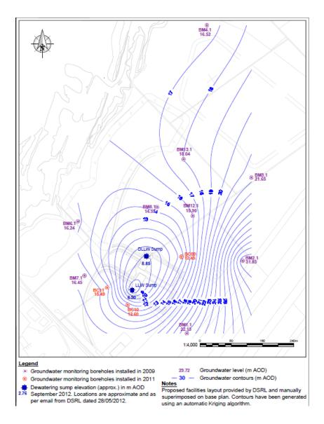
**Figure B-2:** Groundwater levels at the NLLWF site in October 2012, indicating a cone of depression from dewatering the Phase 1 excavations.
