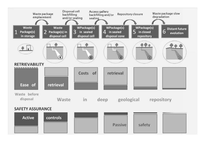
**Figure 2.1:** Graphical description of the R-scale (from NEA, 2011). The figure illustrates the changing degree of retrievability, and passive versus active controls on the waste for the lifecycle stages of a waste package. During the operational phase, not all waste packages in the facility will be at the same lifecycle stage.
