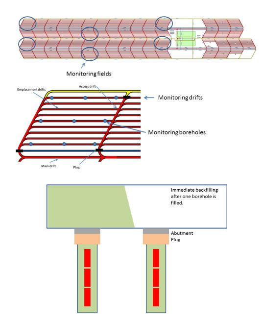
**Figure 5.2:** German clay concept, showing general layout and features, locations where monitoring is expected to take place, and illustration of continuous backfilling. Monitoring drifts are emplacement drifts in which monitoring boreholes (indicated by blue circles) are located.
