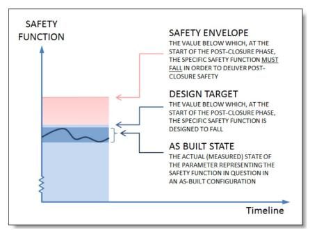
**Figure 3.3:** Visualisation of the general relationship between the safety envelope, the design target and the as-built state for one specific parameter. From IAEA (2016). References to values of safety functions in the figure, refer to values of a parameter representing a safety function.
