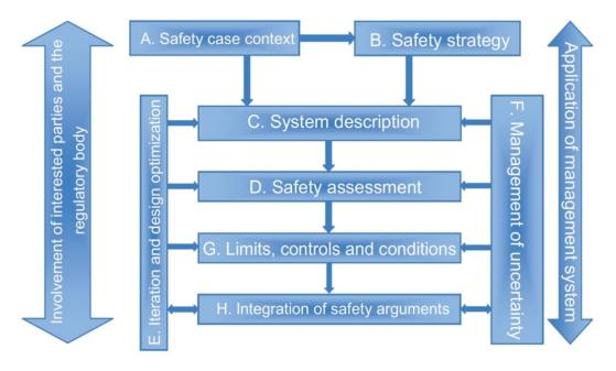
Figure 3.1: Components of a safety case. From IAEA (2012).
