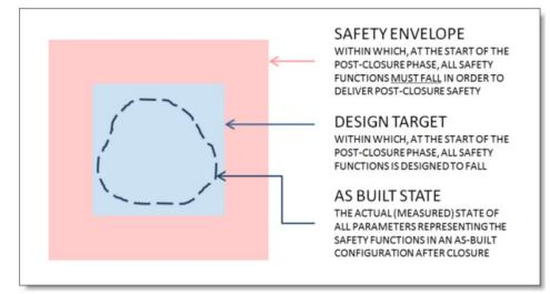
**Figure 3.4:** Visualisation of the general relationship between the safety envelope, the design target and the as-built state for all parameters. From IAEA (2016). References to values of safety functions in the figure, refer to values of a parameter representing a safety function.
