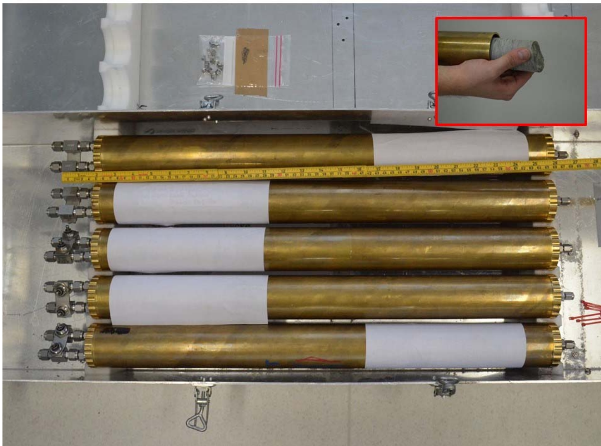
Figure 5. Brass tubes used for inoculation and analysis of gases emitted from porewater in drillcores.
