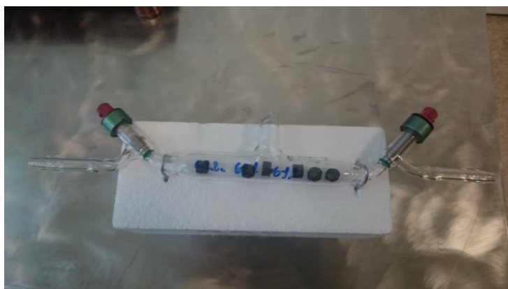
Figure 6: Graphite samples sealed in a glass vessel
