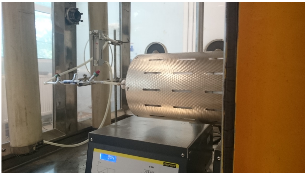
Figure 7: Apparatus for C-14 and H-3 determination release in gas phase
