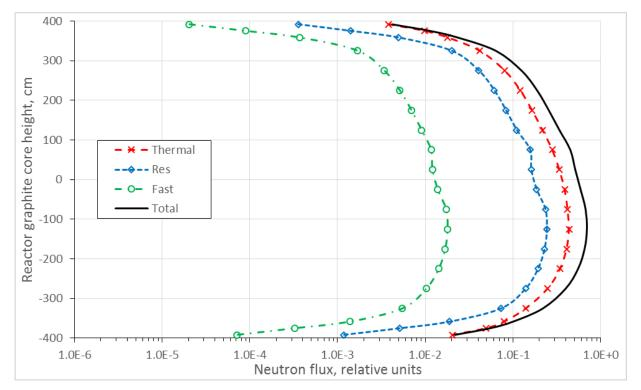
Figure 29: Distribution of neutron flux in graphite columns containing CPS channels (MCR1) in RBMK-1500 reactor at Ignalina NPP Unit 1
