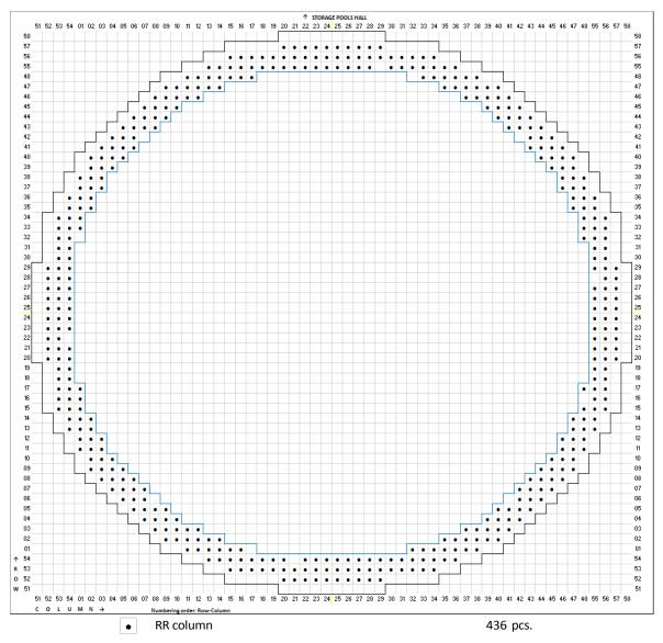
Figure 22: Layout of RR graphite columns containing graphite rods in RBMK-1500 reactor at Ignalina NPP Unit 1
