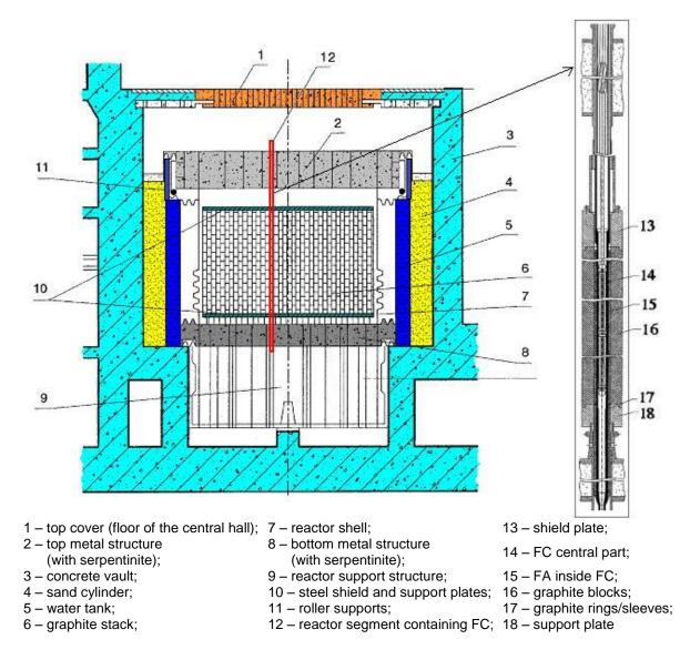
Figure 2: Vertical cross-section of the RBMK-1500 reactor vault (reproduced from [2])
