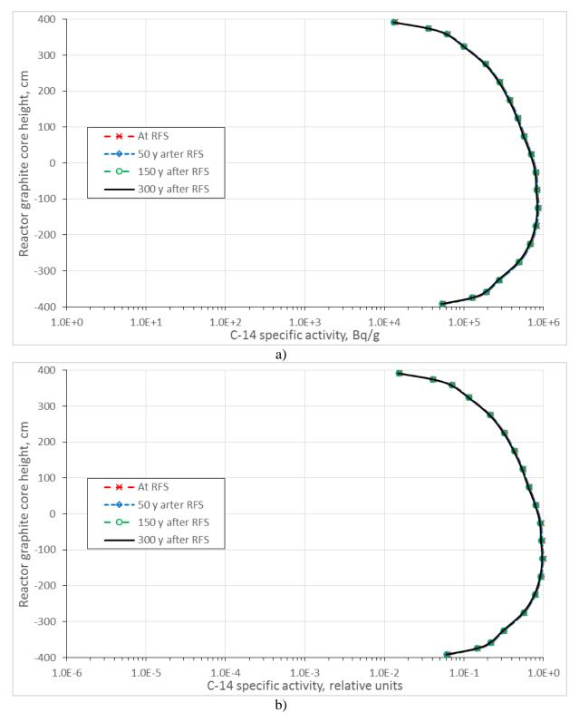
Figure 15: Distribution of absolute a) and normalised b) C-14 specific activity in graphite columns containing fuel channels in RBMK-1500 reactor central part at Ignalina NPP Unit 1
