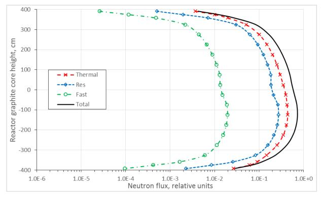
Figure 38: Distribution of neutron flux in graphite columns containing CPS channels (FASR) in RBMK-1500 reactor at Ignalina NPP Unit 1
