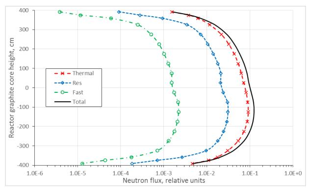
Figure 44: Distribution of neutron flux in graphite columns containing CPS channels (fission chambers) in RBMK-1500 reactor at Ignalina NPP Unit 1
