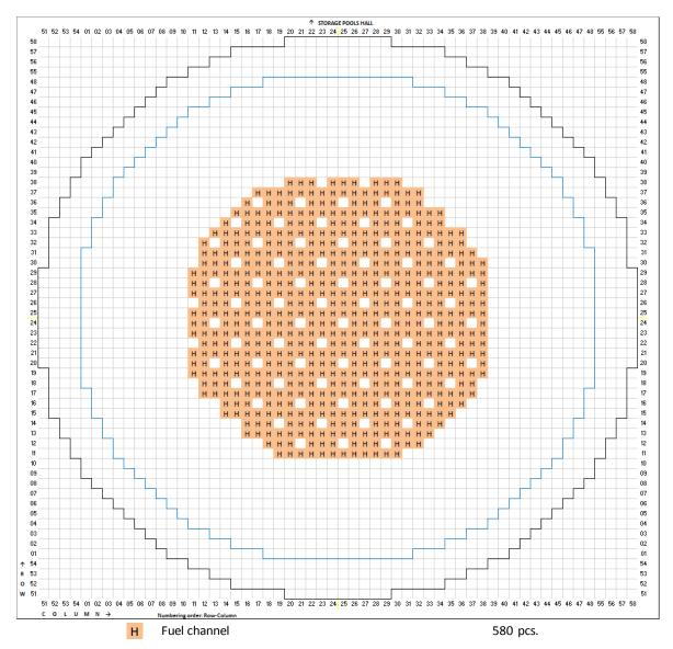
Figure 13: Layout of graphite columns containing fuel channels in RBMK-1500 reactor central part at Ignalina NPP Unit 1
