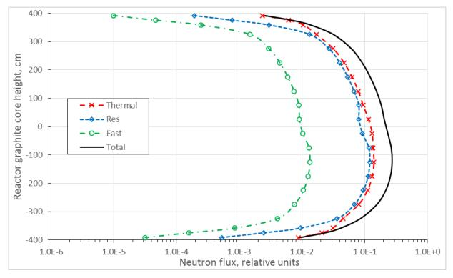
Figure 20: Distribution of neutron flux in graphite columns containing fuel channels in RBMK-1500 reactor second peripheral part at Ignalina NPP Unit 1
