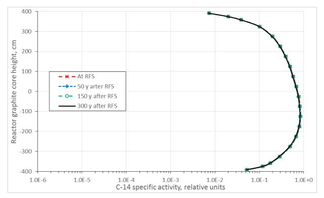
Figure 39: Distribution of C-14 specific activity in graphite columns containing CPS channels (FASR) in RBMK-1500 reactor at Ignalina NPP Unit 1
