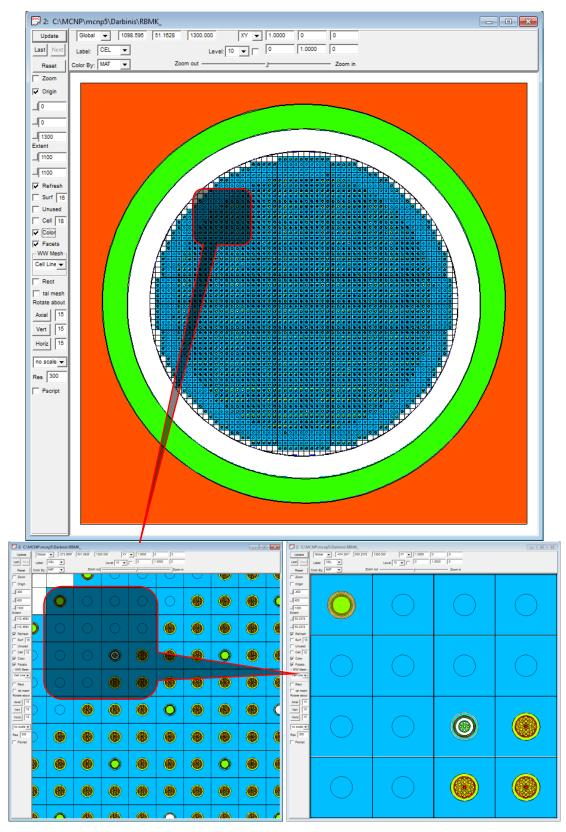
Figure 9: Horizontal cross-section of modelled RBMK-1500 reactor using MCNP
