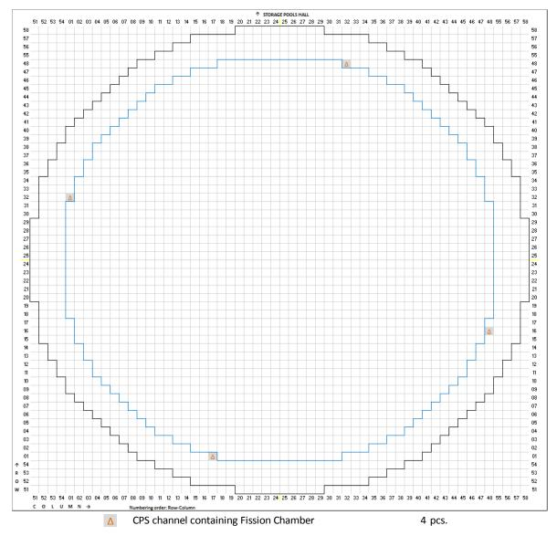
Figure 43: Layout of graphite columns containing CPS channels (fission chambers) in RBMK-1500 reactor at Ignalina NPP Unit 1
