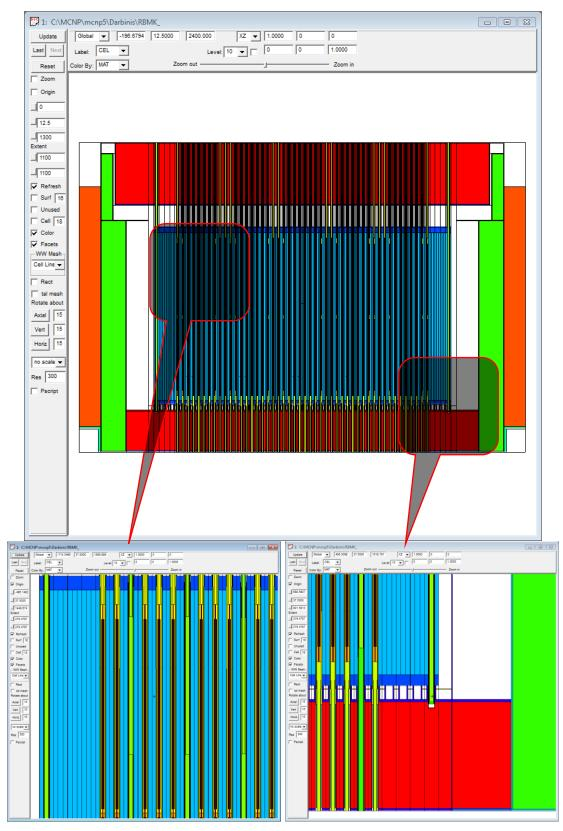
Figure 8: Vertical cross-section of modelled RBMK-1500 reactor using MCNP
