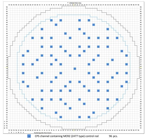
Figure 31: Layout of graphite columns containing CPS channels (MCR2) in RBMK-1500 reactor at Ignalina NPP Unit 1
