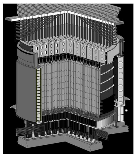
Figure 1: General view of the RBMK reactor [1]
