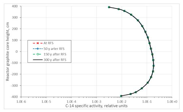
Figure 45: Distribution of C-14 specific activity in graphite columns containing CPS channels (fission chambers) in RBMK-1500 reactor at Ignalina NPP Unit 1
