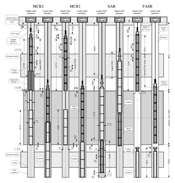
Figure 5: Layout of CPS rods position along the core of RBMK-1500 reactor [4]
