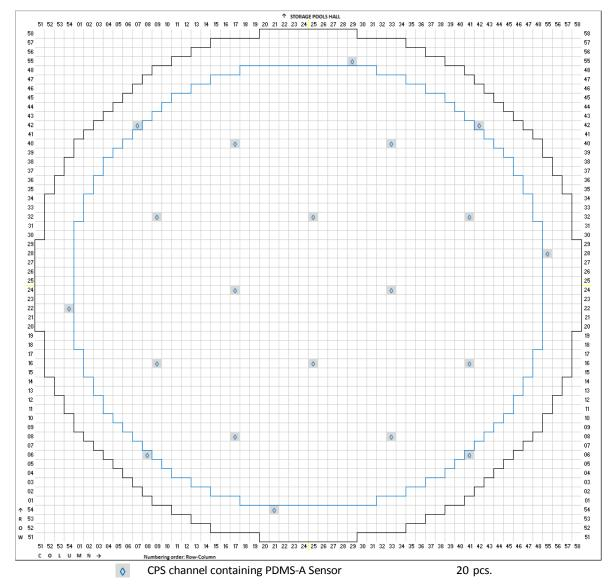
Figure 40: Layout of graphite columns containing CPS channels (PDMS-A) in RBMK-1500 reactor at Ignalina NPP Unit 1
