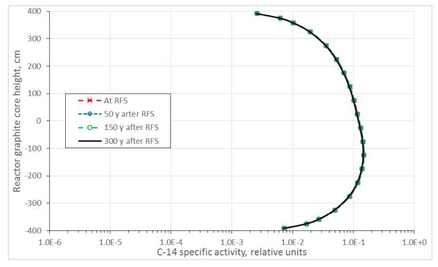
Figure 24: Distribution of C-14 specific activity in RR graphite columns containing graphite rods in RBMK-1500 reactor at Ignalina NPP Unit 1
