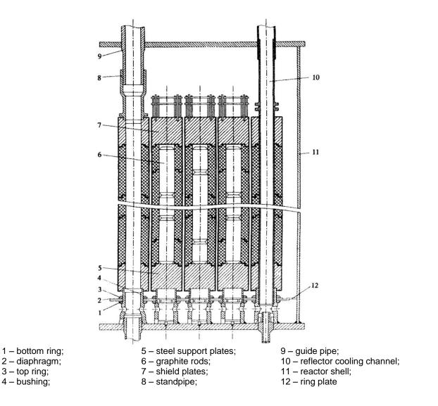
Figure 4: Segment of the reactor core with the part of graphite stack [2]
