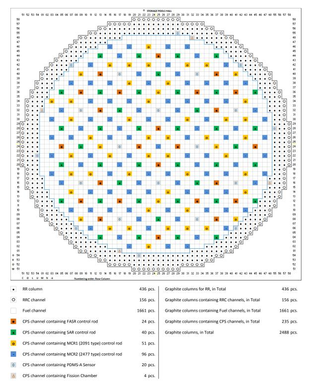
Figure 6: Layout of graphite columns in RBMK-1500 reactor at Ignalina NPP Unit 1
