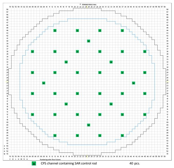
Figure 34: Layout of graphite columns containing CPS channels (SAR) in RBMK-1500 reactor at Ignalina NPP Unit 1
