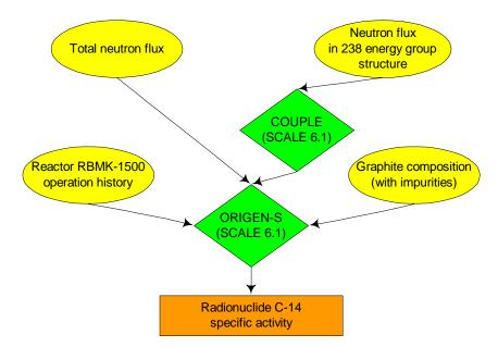
Figure 11: General scheme of C-14 activity modelling in RBMK-1500 reactor graphite core at Ignalina NPP Unit 1
