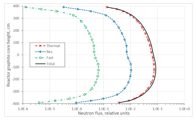
Figure 23: Distribution of neutron flux in RR graphite columns containing graphite rods in RBMK-1500 reactor at Ignalina NPP Unit 1
