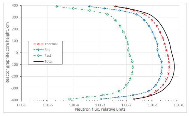
Figure 32: Distribution of neutron flux in graphite columns containing CPS channels (MCR2) in RBMK-1500 reactor at Ignalina NPP Unit 1
