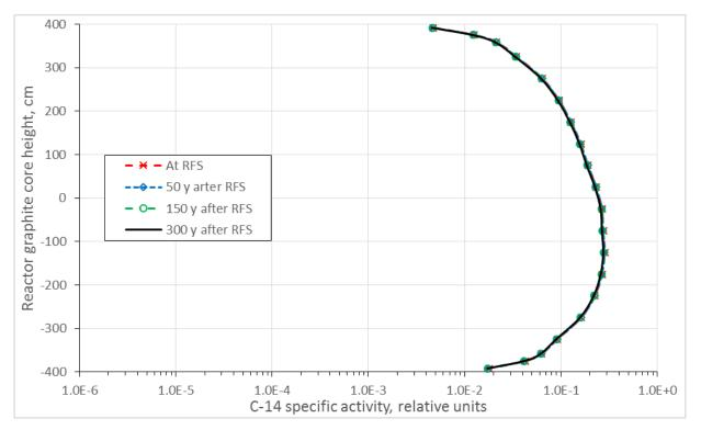
Figure 21: Distribution of C-14 specific activity in graphite columns containing fuel channels in RBMK-1500 reactor second peripheral part at Ignalina NPP Unit 1
