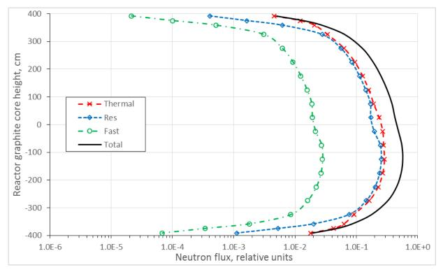
Figure 17: Distribution of neutron flux in graphite columns containing fuel channels in RBMK-1500 reactor first peripheral part at Ignalina NPP Unit 1
