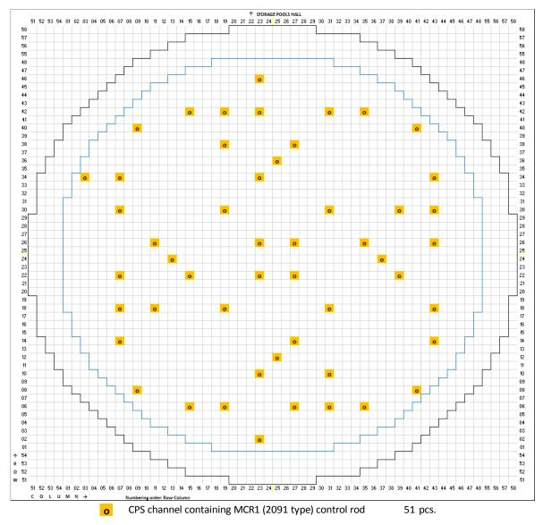
Figure 28: Layout of graphite columns containing CPS channels (MCR1) in RBMK-1500 reactor at Ignalina NPP Unit 1
