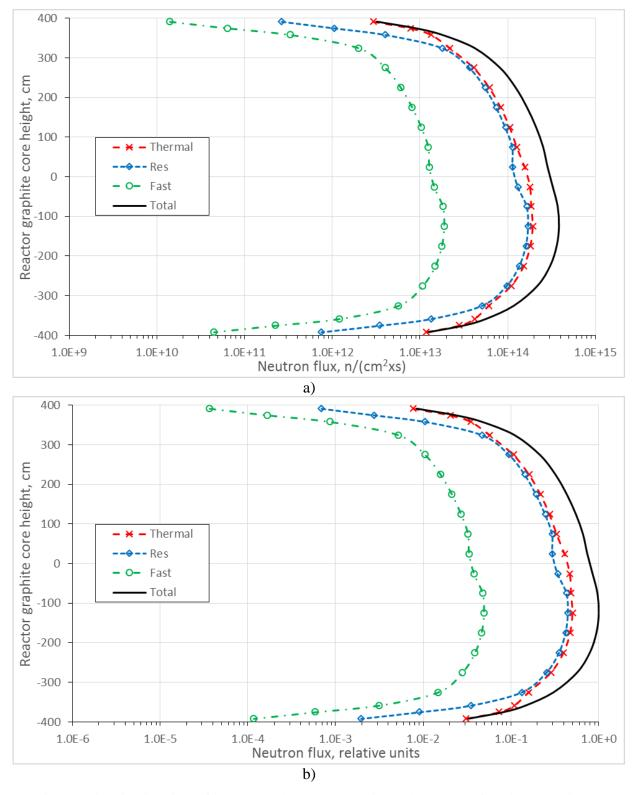
Figure 14: Distribution of absolute a) and normalised b) neutron flux in graphite columns containing fuel channels in RBMK-1500 reactor central part at Ignalina NPP Unit 1
