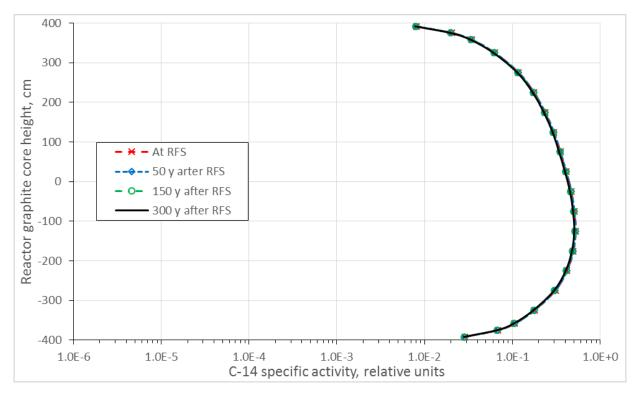
Figure 42: Distribution of C-14 specific activity in graphite columns containing CPS channels (PDMS-A) in RBMK-1500 reactor at Ignalina NPP Unit 1
