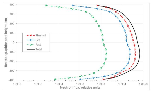
Figure 35: Distribution of neutron flux in graphite columns containing CPS channels (SAR) in RBMK-1500 reactor at Ignalina NPP Unit 1
