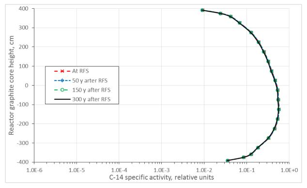
Figure 18: Distribution of C-14 specific activity in graphite columns containing fuel channels in RBMK-1500 reactor first peripheral part at Ignalina NPP Unit 1
