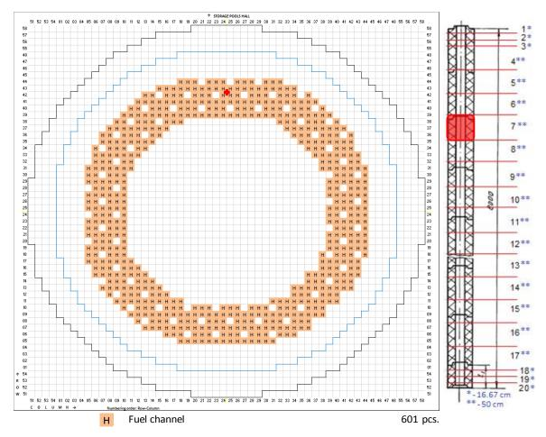
Figure 46: Position of graphite sample taken from the area of graphite columns in RBMK-1500 reactor first peripheral part at Ignalina NPP Unit 1
