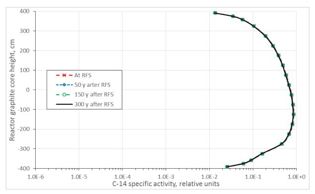
Figure 36: Distribution of C-14 specific activity in graphite columns containing CPS channels (SAR) in RBMK-1500 reactor at Ignalina NPP Unit 1
