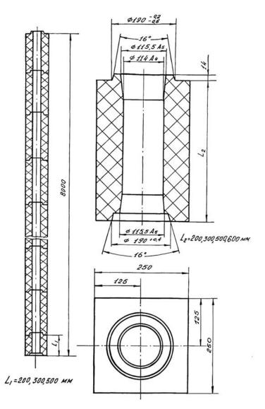
Figure 3: Schematic view of graphite column and block of RBMK-1500 reactor [3]
