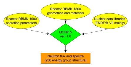
Figure 7: General scheme of neutron flux modelling in RBMK-1500 reactor graphite core at Ignalina NPP Unit 1
