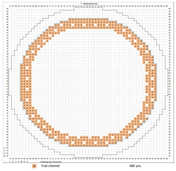
Figure 19: Layout of graphite columns containing fuel channels in RBMK-1500 reactor second peripheral part at Ignalina NPP Unit 1
