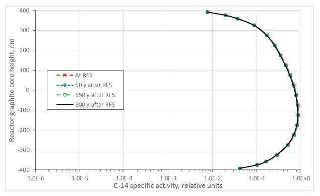
Figure 30: Distribution of C-14 specific activity in graphite columns containing CPS channels (MCR1) in RBMK-1500 reactor at Ignalina NPP Unit 1
