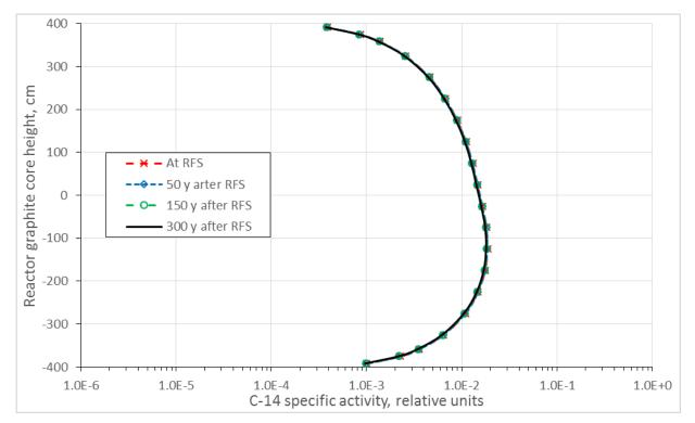
Figure 27: Distribution of C-14 specific activity in graphite columns containing RRC channels in RBMK-1500 reactor at Ignalina NPP Unit 1
