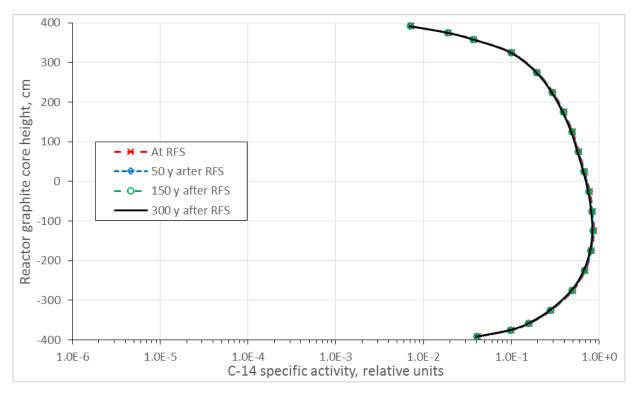
Figure 33: Distribution of C-14 specific activity in graphite columns containing CPS channels (MCR2) in RBMK-1500 reactor at Ignalina NPP Unit 1
