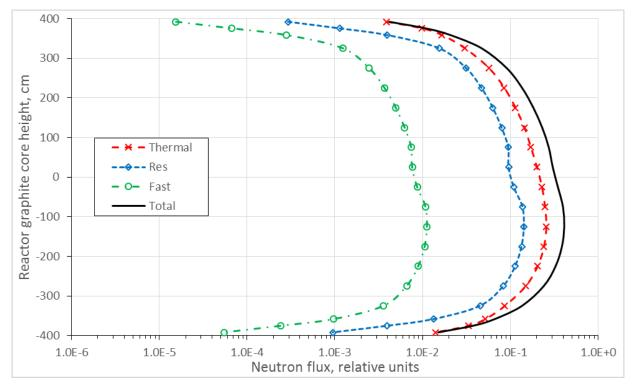
Figure 41: Distribution of neutron flux in graphite columns containing CPS channels (PDMS-A) in RBMK-1500 reactor at Ignalina NPP Unit 1
