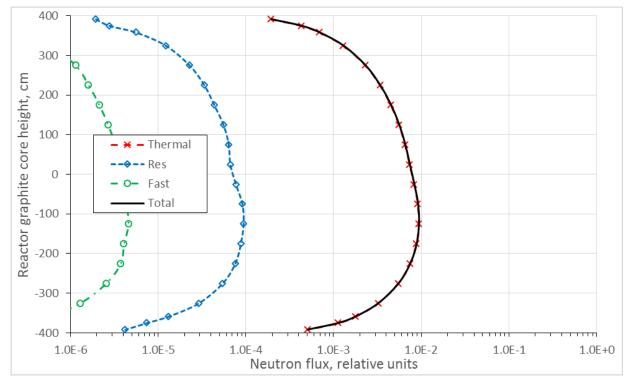
Figure 26: Distribution of neutron flux in graphite columns containing RRC channels in RBMK-1500 reactor at Ignalina NPP Unit 1
