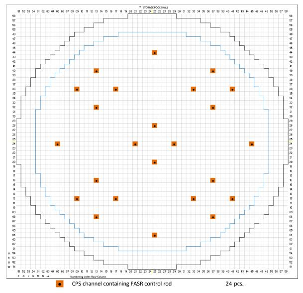
Figure 37: Layout of graphite columns containing CPS channels (FASR) in RBMK-1500 reactor at Ignalina NPP Unit 1
