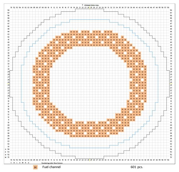
Figure 16: Layout of graphite columns containing fuel channels in RBMK-1500 reactor first peripheral part at Ignalina NPP Unit 1
