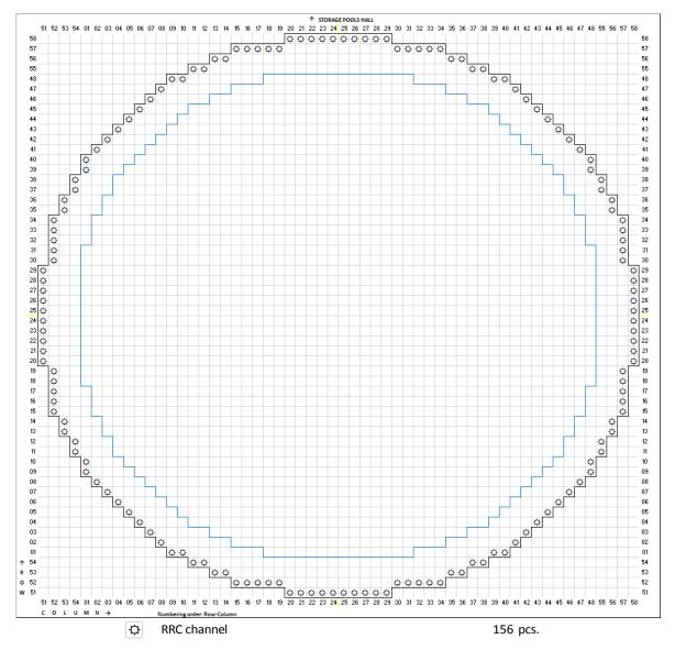
Figure 25: Layout of graphite columns containing RRC channels in RBMK-1500 reactor at Ignalina NPP Unit 1
