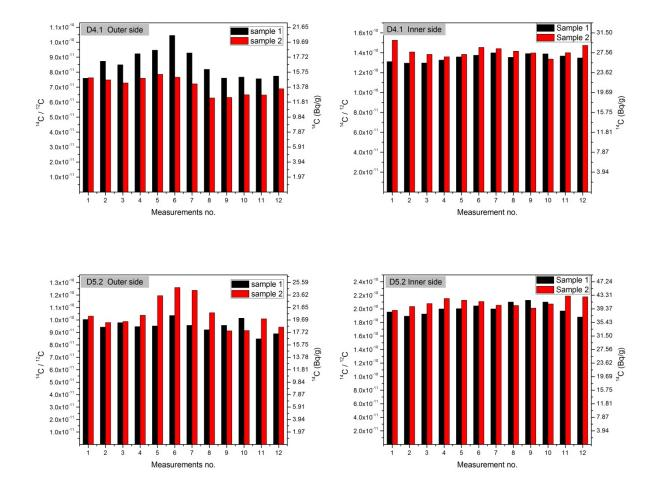
Figure 16: Statistics of AMS measurement for the analyzed samples (results for sample 6-2 are not shown, as they are unreliable).
