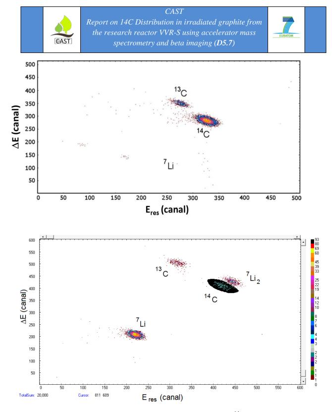
Figure 9: Two bi-parametric spectra showing the <sup>14</sup>C concentration.
