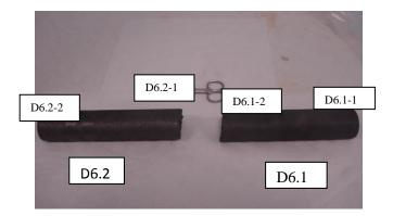
Figure 5: Irradiated graphite samples collected from small rod in disc 6
