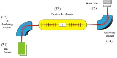
Figure 7: Schematic diagram of an AMS- facility
