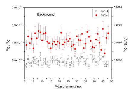
Figure 15: Background radiocarbon concentration measured from blank samples
