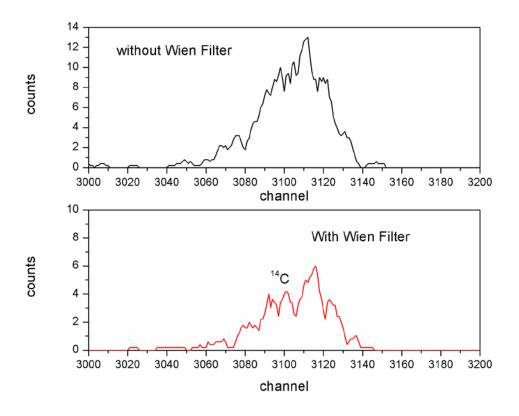
Figure 18: <sup>14</sup>C spectra at the 9 MV tandem accelerator.
