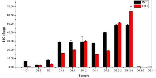
Figure 13:Results of the AMS experiments determining the <sup>14</sup>C concentration<br/>accumulated in the thermal column of the VVR-S reactor
