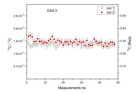
Figure 14: AMS results of the standard sample (OXA II) used in this experiment
