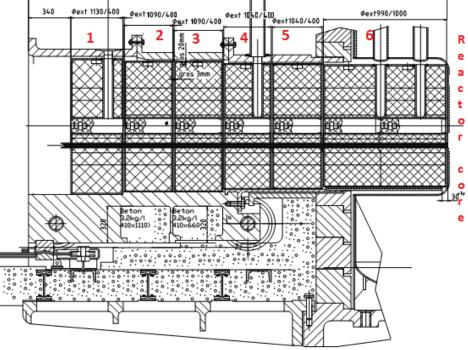
Figure 6: VVR-S thermal column cross section
