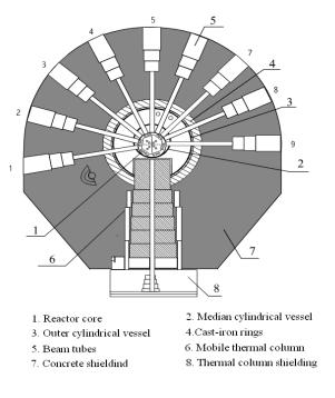
VVR-S REACTOR HORIZONTAL CROSS-SECTION
