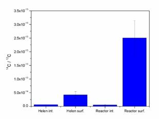
Figure 10: The <sup>14</sup>C concentrations measured from samples of unirradiated graphite as used in the subcritical assembly *Helen* and the VVR-S reactor
