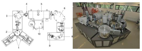
Figure 8b: Left: the general layout of 1 MV HVEE AMS facility in Bucharest, Romania. Right: photograph of the facility.
