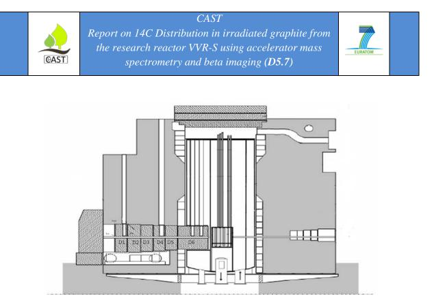
Figure 2: Vertical cut-view through the VVR-S reactor and the movable thermal column with its 6 discs
