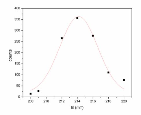
Figure 17: Determination of the optimum magnetic field setting for the Wien Filter
