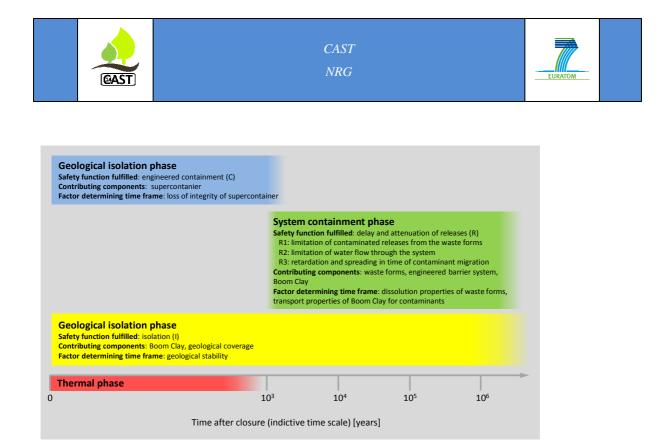
Figure 5. Safety functions provided by the main components of the disposal system in Boom Clay and its geological coverage
