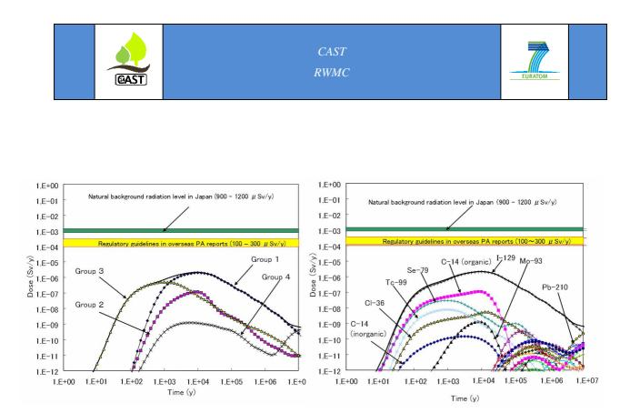
Figure 8: Results of dose assessment for each waste group (left) and for each radionuclide (right).
