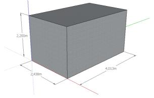
Figure 1: Steel container considered for the analysis of C-14 migration from RBMK-1500 graphite waste
