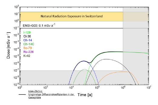
Figure 4. Dose curve calculated for an HLW repository in the siting region Zurich Northeast, Alternative Case 'Unfavourable Diffusion Coefficients' (NAGRA, 2014a,e). Ch-14 = organic <sup>14</sup>C IRF, Ch-14C = organic <sup>14</sup>C CR
