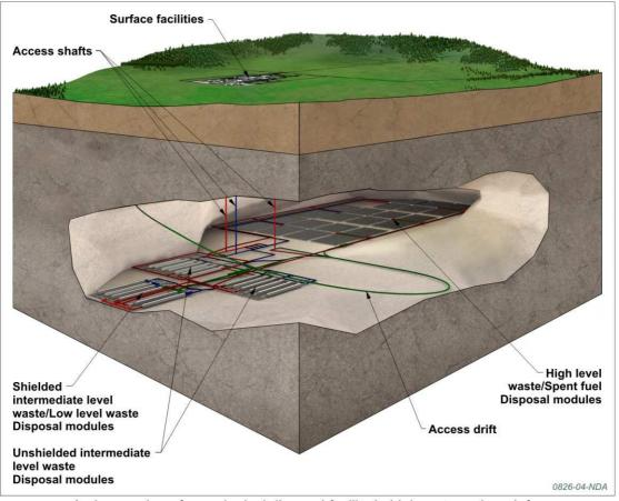
An impression of a geological disposal facility in higher strength rock for higher activity radioactive waste
