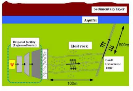
Figure 5: Overview of radionuclide transport pathway.
