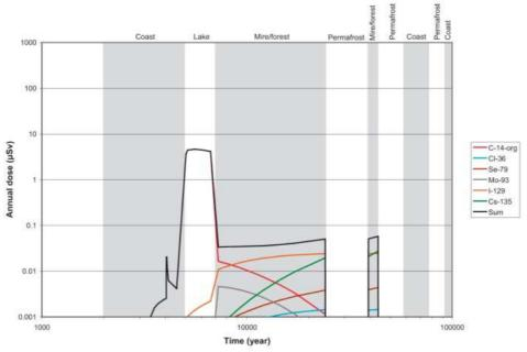
Figure 1-3. Calculated doses from the Silo in SAR-08 [SKB2008]. To the left doses from the main scenario. To the right doses from the gas driven advection scenario.
