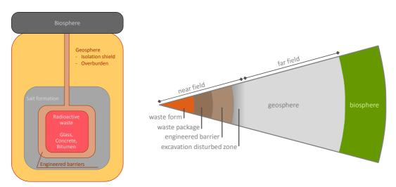
Figure 4. Principle of a multi-barrier system in salt formations (left), and in Boom Clay (OPERA, right)
