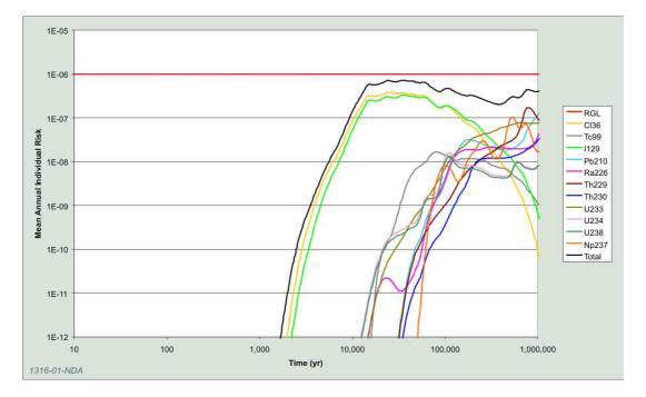
Figure 6 Reference case mean radiological risk against time for key radionuclides for ILW and LLW [22]
