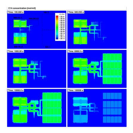
Figure 5: Example of a possible evolution with time of concentration of carbon 14 at repository level (2009 repository architecture)
