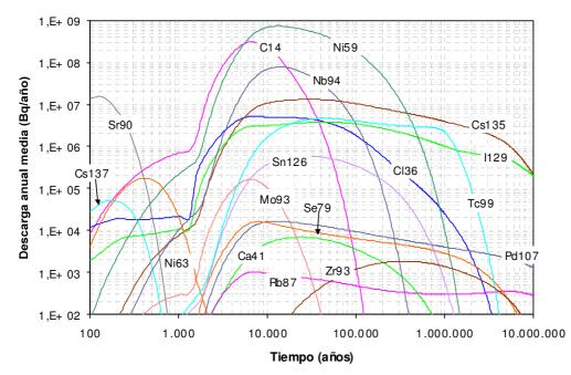
Figure - Mean Release Rates from the near field in the probabilistic calculations (reference scenario). Fission and activation products.Fig 6-17 de Enresa, 2000.
