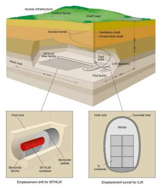
Figure 1. Conceptual outline of a deep geological repository for SF/HLW and ILW (NAGRA 2008b, modified)
