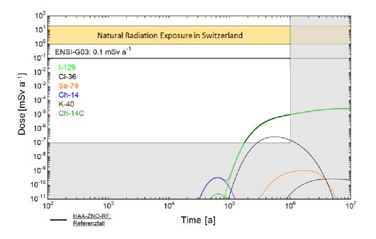
Figure 3. Dose curve calculated for an HLW repository in the siting region Zurich Northeast, Reference Case (NAGRA, 2014a,e). Ch-14 = organic <sup>14</sup>C IRF, Ch-14C = organic <sup>14</sup>C CR
