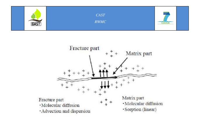
Figure 7: Conceptual illustration of the radionuclide transport in the natural barrier (host rock).
