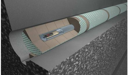
Figure 1: Visualisation of the Czech DGR concept using horizontal boreholes
