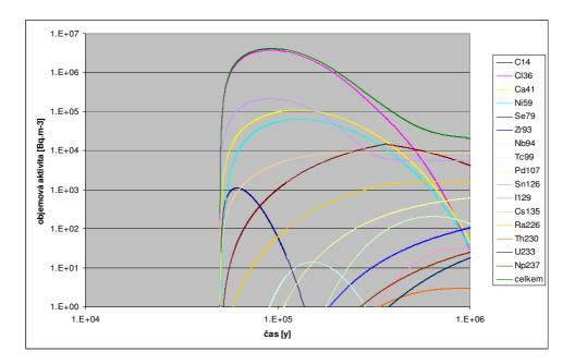
Figure 4: Release of radionuclides form source term to geosphere
