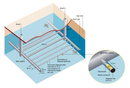
Figure 2 Concept for the disposal in rock salt in the Netherlands
