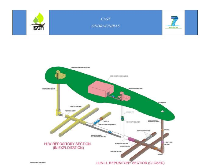
Figure 1 Reference design for the disposal of category B and C waste in Belgium
