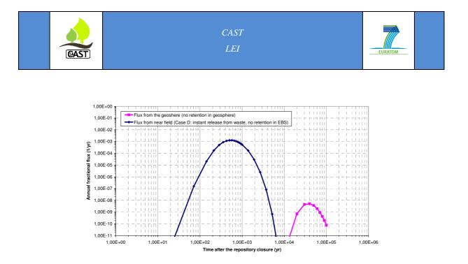
Figure 7: Release of C-14 from the backfill and geosphere
