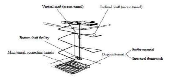
Figure 2: Basic concept for the TRU repository in Japan.
