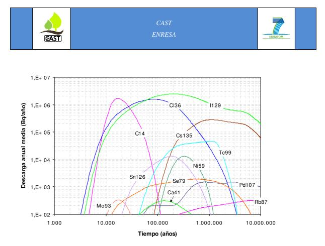
Figure - Mean Release Rates from the geosphere in the probabilistic calculations (reference scenario). Fission and activation products.Fig 6-19 de Enresa2000.
