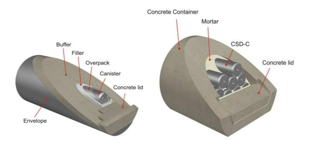
Figure 2. Example of a supercontainer and a monolith design for vitrified HLW canisters and compacted waste ('CSD-C'), respectively.
