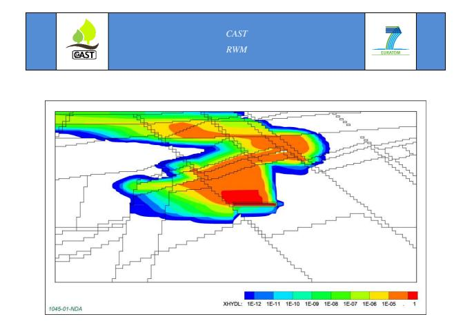
Figure 5 Contour plot of mass fraction of dissolved gas at 240 years post-closure for gas migration from a GDF in a higher strength rock [17].
