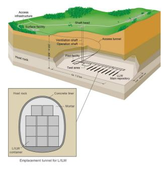
Figure 2. Conceptual outline of a deep geological repository for L/ ILW (NAGRA 2008b, modified)
