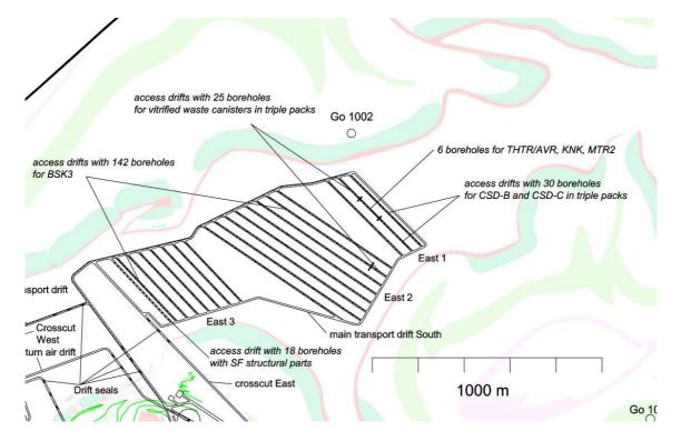
Figure 2: Layout of the north-eastern part of the repository [Bollingerfehr et al. 2012]
