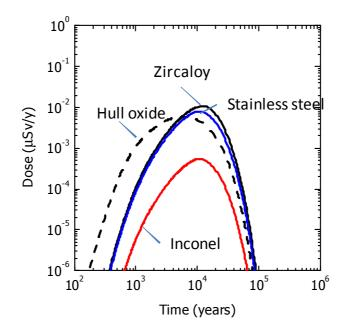
Figure 9: Results of dose assessment from respective components of hull waste. The detailed data are obtained from Sakuragi et al. [SAKURAGI et al., 2013].
