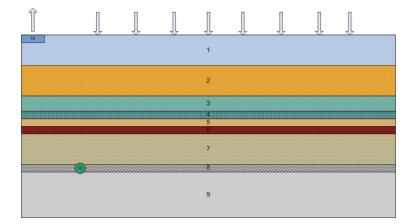
Figure 4: Far field model (1 – glacial loam, 2 – sand, 3 – anhydrite, 4 – limestone, 5 – sandstone, 6 – clay, 7 – sandstone, 8 – weathered crystalline rocks, 9 – monolithic crystalline rocks, 10 – groundwater discharge area, 11 – radionuclide flux from the crystalline rock)
