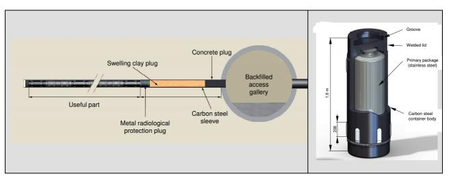
Figure 3: Schematic illustration of the design for HL waste disposal cell (left) and HL waste package (right)
