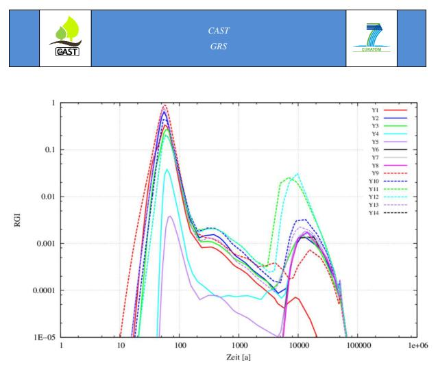
Figure 3: RGI resulting from the C-14 flux out of the spent fuel containers calculated at the isolating rock zone boundary for different variants [Larue et al. 2013]
