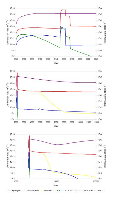
Figure 3 Gas generation from the 2004 UILW inventory for the Reference case – plotted on various time scales. The bulk gases (i.e. H2 and CH4) are plotted vs. the left-hand axis, and the active gases (i.e. 3HH, 14CH4 and 222Rn) are plotted vs. the right-hand axis. CO2 reacts with cement [9].
