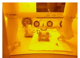
Leaching vessel for irradiated stainless steel in hot cell (courtesy of NRG)
