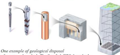
One example of geological disposal of spent nuclear fuel: The Swedish KBS-3 method
