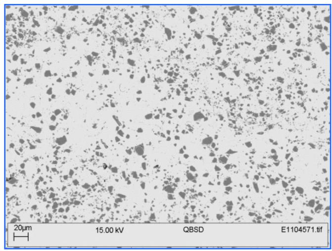
20 vol% B<sub>4</sub>C in an aluminium matrix
