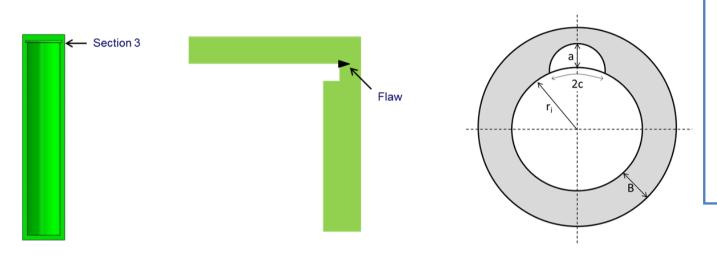
10-mm-deep hemispherical flaws located circumferentially at either the inner or outer surface of the final closure weld or radially in base of container in region of high tensile stress
