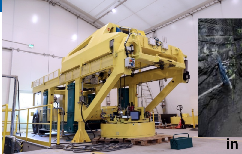
Buffer installation machine
