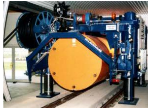
Emplacement Technique for POLLUX-Casks
