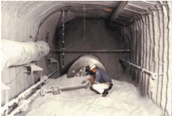
In situ-Heating Test (10 years) to Proof POLLUX-Cask Emplacement Concept
