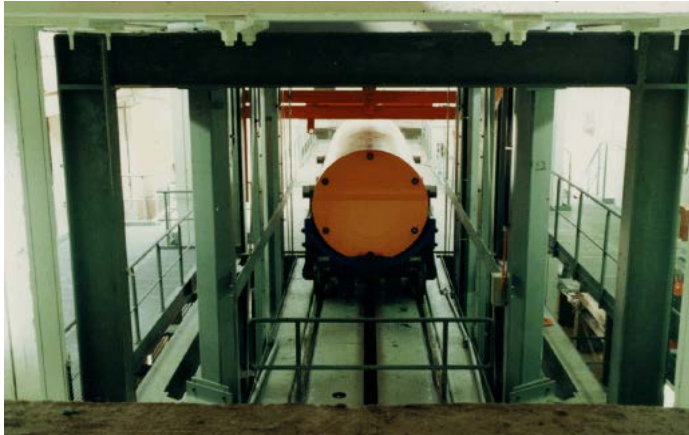
Shaft Transport system for Payloads up to 85 t
