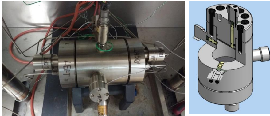
Fig. 3. Representation of the new designed oedometer cell at constant volume: (a) schematic layout, (b) cell with upper piston unscrewed into load frame and (c) cell with upper piston screwed and installed into X-ray tomograph.
