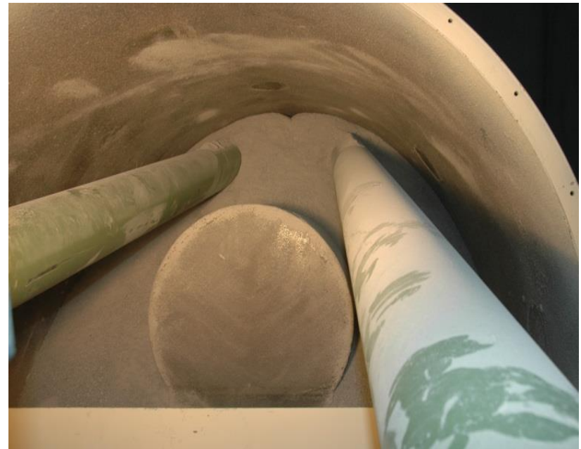
Emplacement of bentonite granulate
