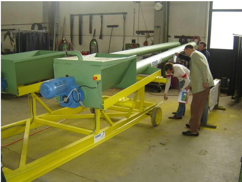
Experimental setup of auger system
