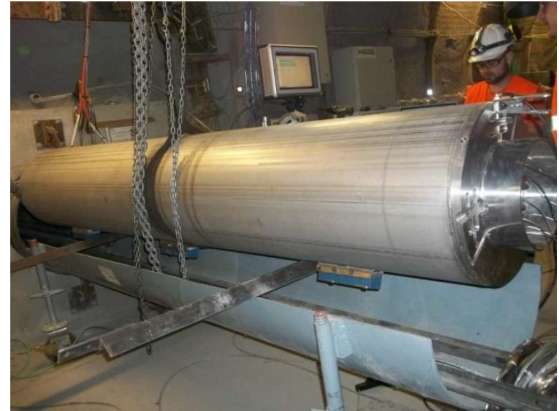
Photo of the heater element used
