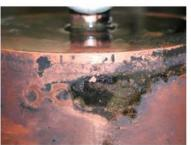
A copper mini-canister that has been exposed to vivid microbial sulphide formation from sulphate, possibly with H<sub>2</sub> from the corroding cast iron insert as the electron donor. See the report **SKB-Technical Report-12-09** for details.
