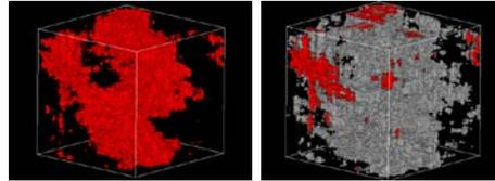
(a) Pore image (b) Pore and C-S-H (C-S-H contain fine pore)
