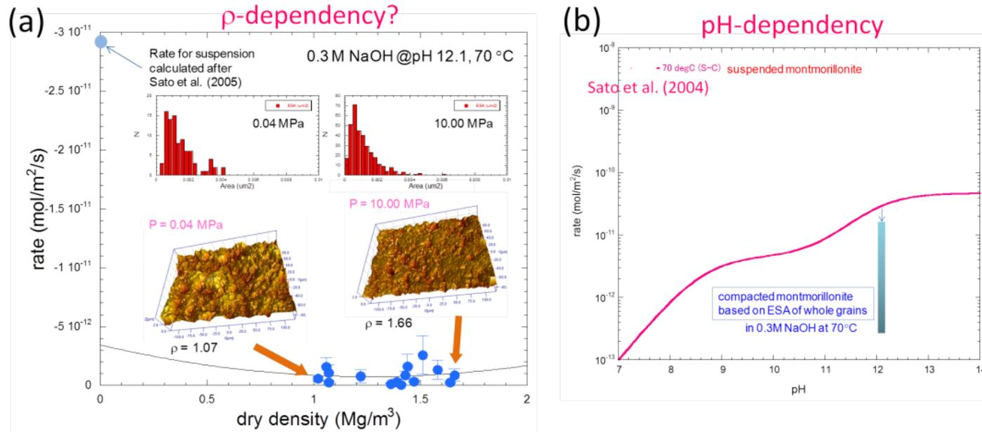
Fig. 11 Plots of dry density vs. rate at 0.04 to 10.00 MPa compaction (a) and pH vs. rate (b).
