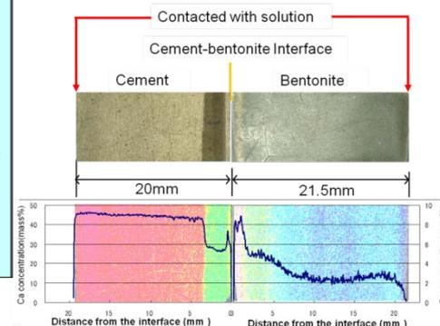
Cross section of the cement block-compacted bentonite interface and Ca concentration profile in the specimen
