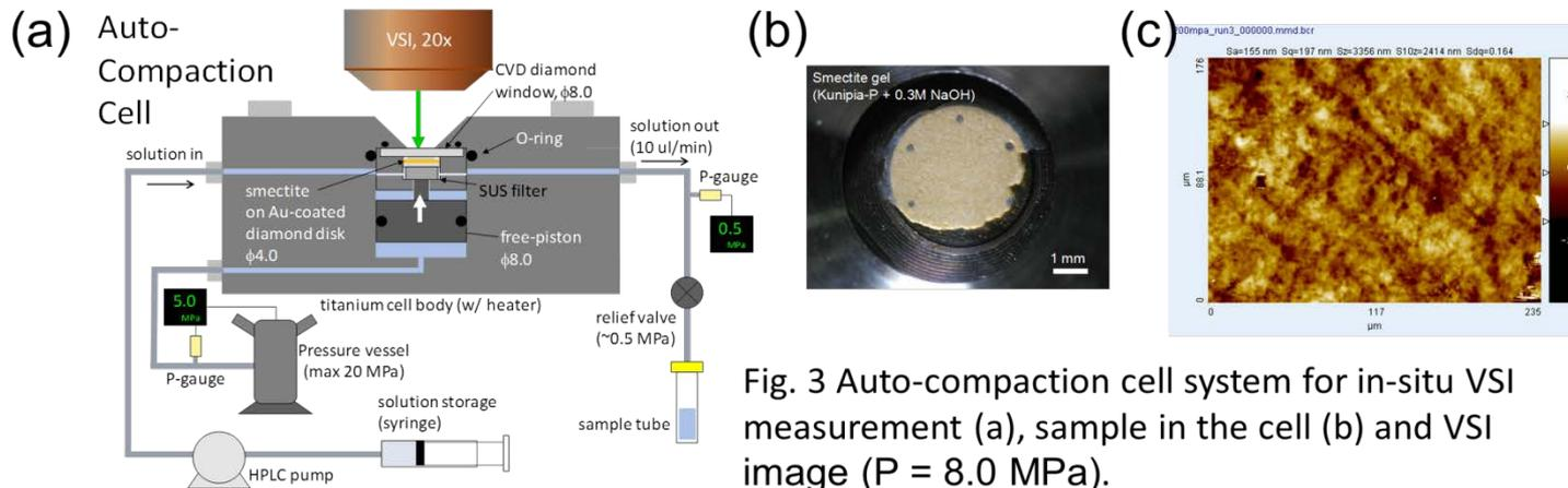
Fig. 3 Auto-compaction cell system for in-situ VSI measurement (a), sample in the cell (b) and VSI image (P = 8.0 MPa).
