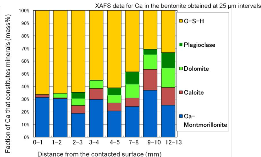
Fraction of Ca that constitutes minerals based on pattern fitting of XAFS data of the homogeneous specimens
