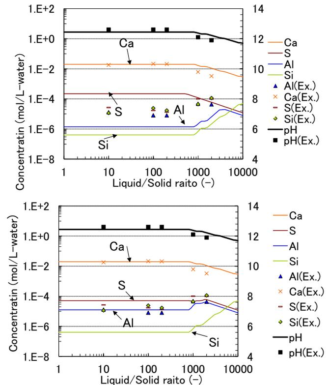
Figs.1 Analyzed (dots) and calculated (lines) liquid composition for OPC with Case 1 (A) and Case 2 (B).
