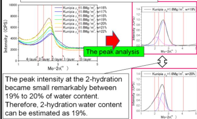
The peak intensity at the 2-hydration became small remarkably between 19% to 20% of water content. Therefore, 2-hydration water content can be estimated as 19%.
