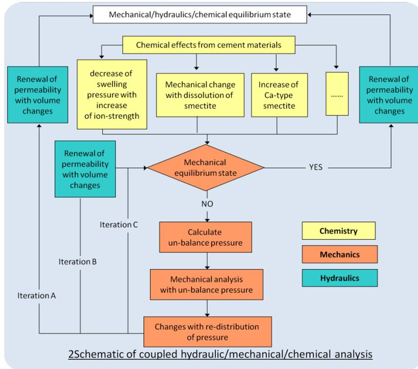
Although iteration A of the coupling method has a stronger effect, the computation time is very long. Therefore, in this study we considered the effect on the evaluation of long term alteration caused by use of **Iteration C**.
