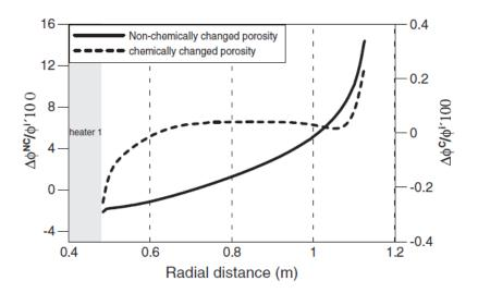
**Example:** Computed changes in porosity due to mechanical and chemical processes in the FEBEX in situ test
