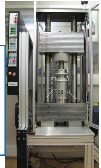
Press « Phenix » pilot operated in axial stress and displacement equipped with φ 120 mm vessel
