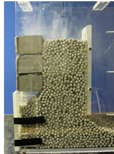
Example of heterogenous bentonite materials : visual mock-up for demonstration of a cut off filling
