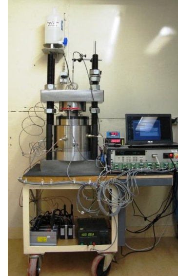
φ 240 mm device developed for studying FSS pellets mixture
