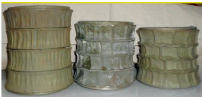
Examples of HIP containers produced during the NNL trials
