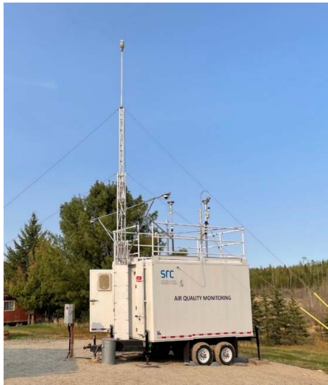
Figure 7-2: Photo Showing the Main Site Study Area (SSA) Atmospheric Monitoring Trailer.
