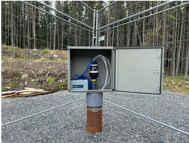
Figure 7-1: Installed shallow groundwater monitoring well in the Wabigoon Lake Ojibway Nation and Ignace Area.
