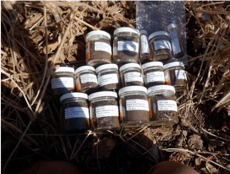
Figure 7-7: Surficial Soil Samples in Laboratory Supplied Containers, September 2024.
