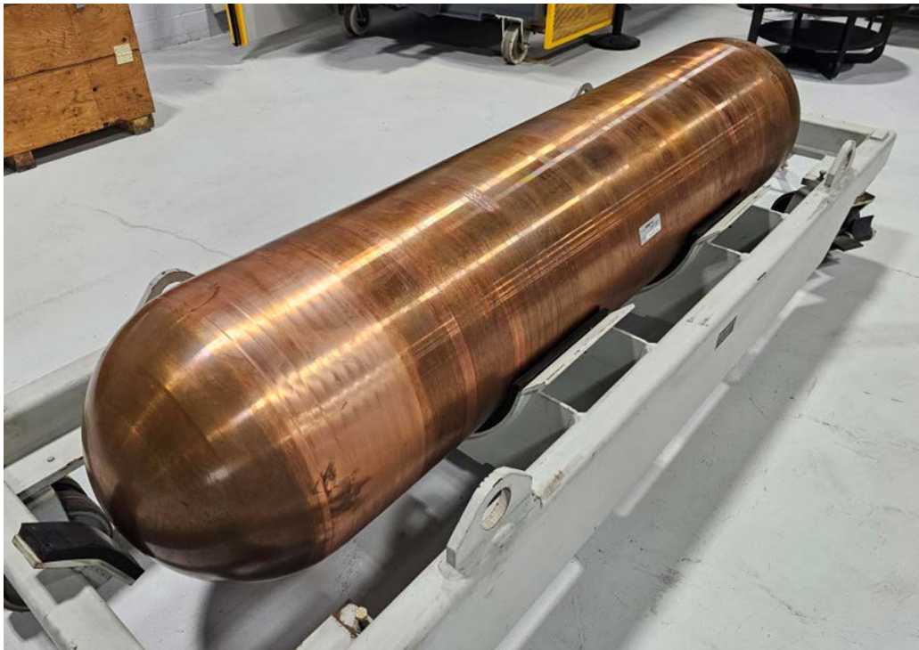
Figure 4-3: Assembled Mark II Used Fuel Container Reference Design
