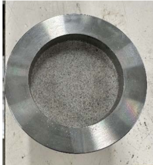
(c) Compacted bentonite-LHHPC in the cell
