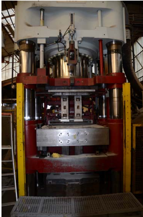
Fig.4.3.1. Uniaxial compaction device and block production (MPC LAVIOSA group, Limay, France).
