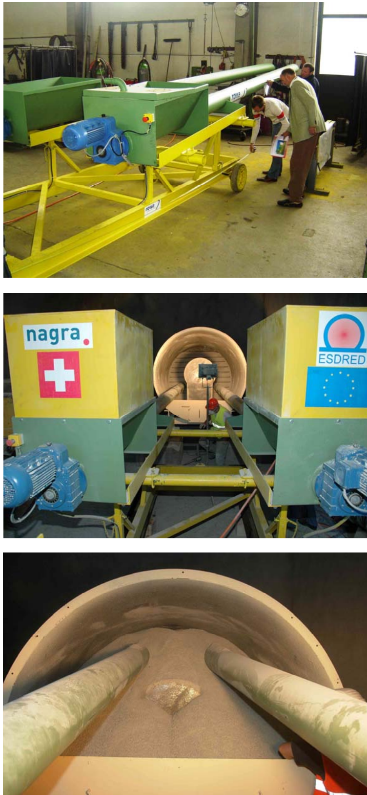
Fig. 4.3.5. Twin auger system for the ESDRED Project (Photos: Nagra).
