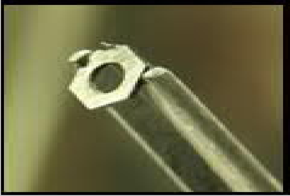
Picture of one of the two activated steel nuts specimens placed in the gas-tight reactor for the corrosion experiment.
