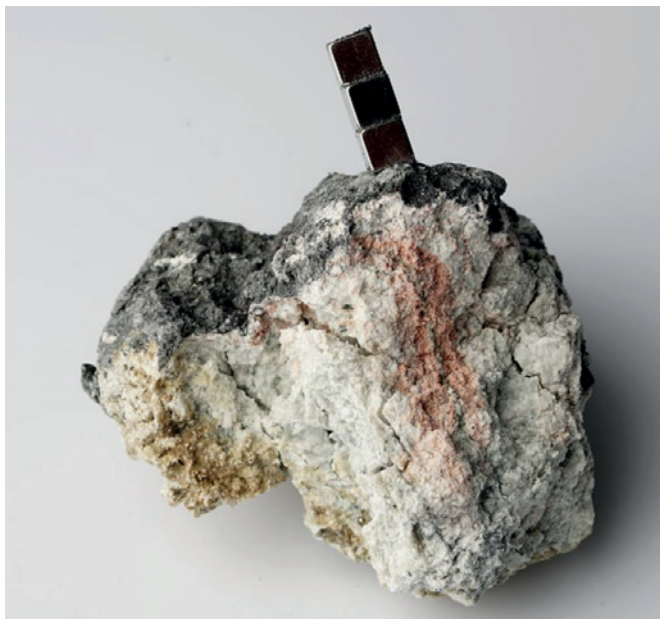
Smectite-magnetite interface, courtesy of SKB
