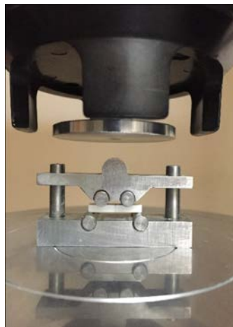
Samples 4x3x20 mm 3 4 point bending tests
