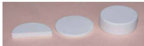
Aluminosilicate ceramic disk of 40 mm diameter and 5, 10 and 22 mm thickness
