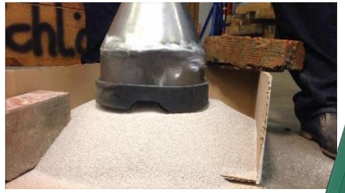
Suction device for sand removal (same dimensions as canister, circulating airflow inside borehole), first pilot tests for air intake
