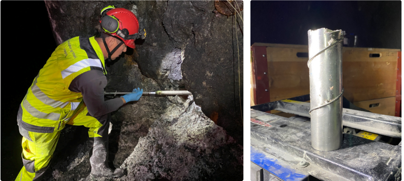
Fig. 6: Sampling of altered clay zones at 1100 m depth in the Kiruna mine (left), specially designed drill bits for sampling (to prevent exposure of the material until it reaches the laboratory) (right).
