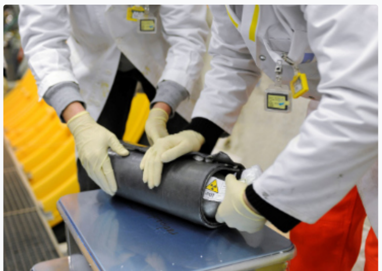
Fig. 6: Handling of a flask containing a radionuclide cocktail prepared by KIT for the CFM experiment. © Comet Photoshopping GmbH, Dieter Enz.
