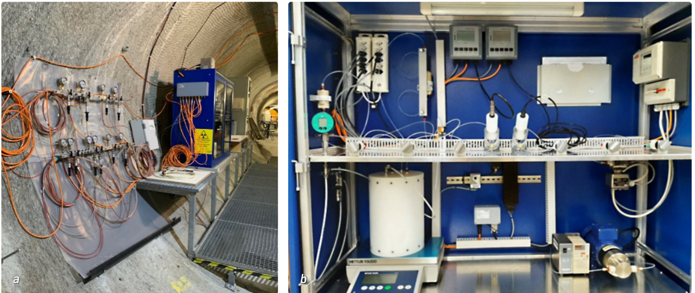
Fig. 2 a, b: CIM surface cabinet. The radionuclides are contained in the white tank in the bottom left of the photograph.
