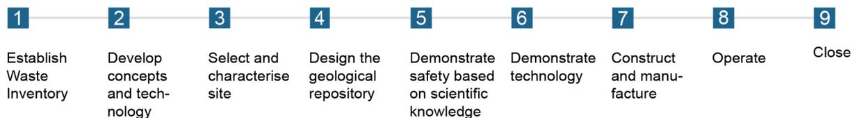
**Figure 3.1:** Main stages in the implementation of geological disposal. The number of the required main, and detailed sub-stages, may be subject to licensing according to the national legislation in question [22].
