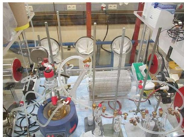
*Dissolution of Zircaloy-4 sample (on the left) and CO<sub>2</sub> absorption apparatus including catalytic furnace (on the right) (courtesy of Karlsruhe Institute of Technology)*
